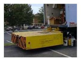
Figure 6-5: Energy Absorption Barrier
