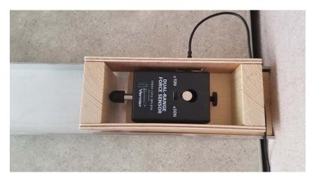
Figure 6-7: Track Loaded with a Force Sensor
